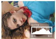
The LCD monitor can be used to display a histogram of any image you take, graphically showing brightness or RGB color distribution among pix-
